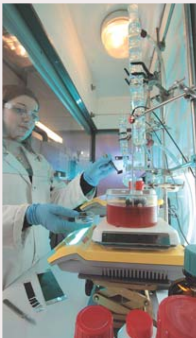
Leaching of Li-ion battery components.
