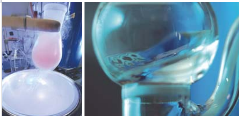
Left: freezing a solution containing a fluorescent chelating agent. Right: agitation of a chemical reactor during the synthesis of peptides on a solid medium.
