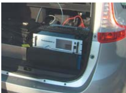
On-board CRDS (Cavity Ring Down Spectroscopy) device for in situ analysis of gas pollutants. This is a system developed by the Physico-Chemistry Department (DPC) located in the CEA Saclay Center, in collaboration with the Université Joseph Fourier of Grenoble.
