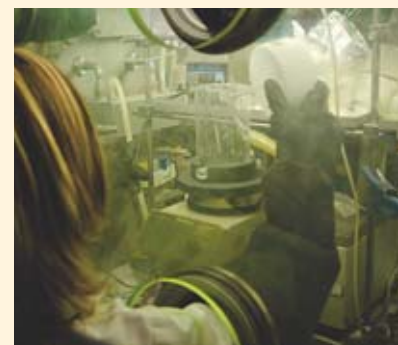
Preparation of an oxalic coprecipitation test in laboratory L15 at ATALANTE for modeling of the process.
