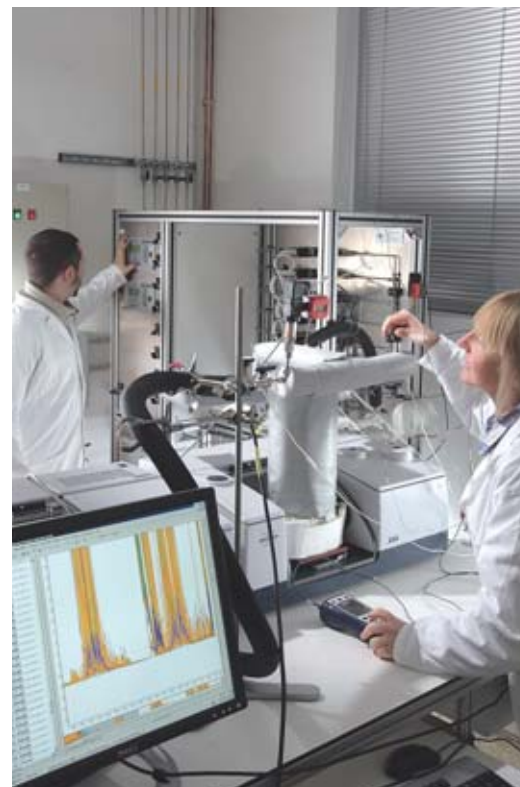
Fourier Transform Infrared spectroscopy (FTIR) analysis facility for measuring traces of inorganic compounds and tars in the synthesized gas.
