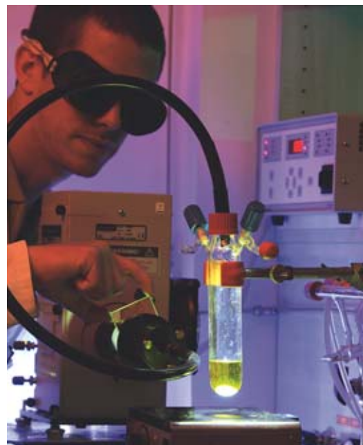
Experiment to photoproduce hydrogen in homogeneous phase catalyzed by the supramolecular complex described in figure 5.
