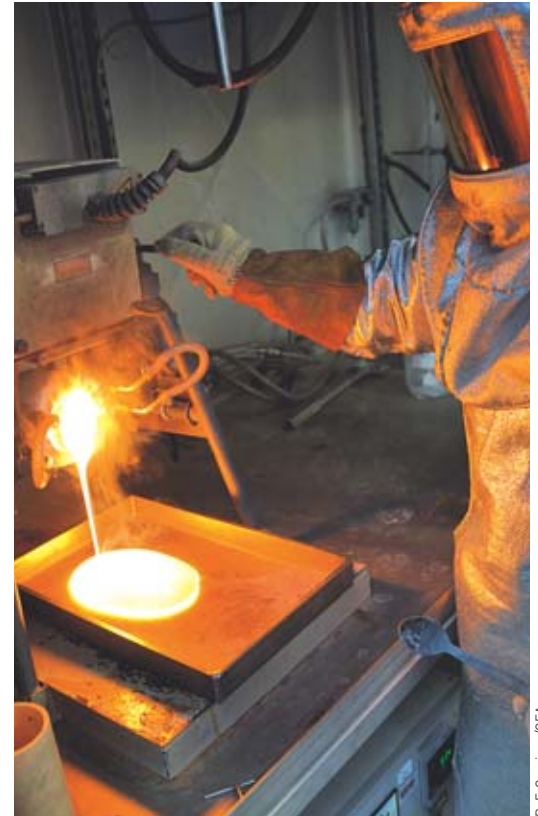
Production by fusion of a waste containment glass for study of its long-term behavior.
