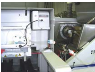
Coupling of a capillary electrophoresis (CE) device (left) with the ICPMS (Inductively Coupled Plasma Mass Spectrometry) device (right).
