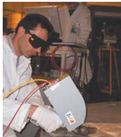
LIBS (Laser Induced Breakdown Spectroscopy) fiber optic device for analysis of elements, marketed by CEA's IVEA start-up.
