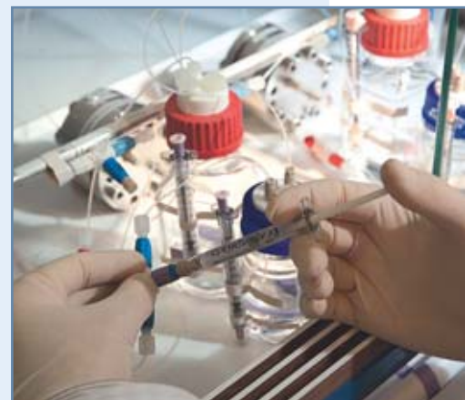
Schematic of a “through” diffusion cell. Left: the sample is “sandwiched” between two tanks into which the tracer is injected (upstream tank) and, in the downstream tank, the quantity of tracer which passed through the sample is measured versus time. Right: injection of the tracer solution into the diffusion cells upstream tank.
