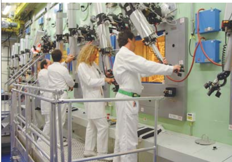
View of the CBP (shielded process chain) in the ATALANTE facility at CEA/Marcoule, where experiments and technical feasibility demonstrations are carried out on the various actinide separation concepts developed.
