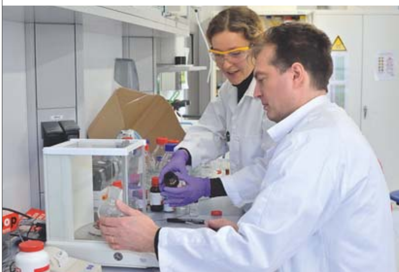
Preparation of radiopharmaceuticals: collection and weighing of a sample for synthesis (Service hospitalier Frédéric-Joliot/SHFJ).
