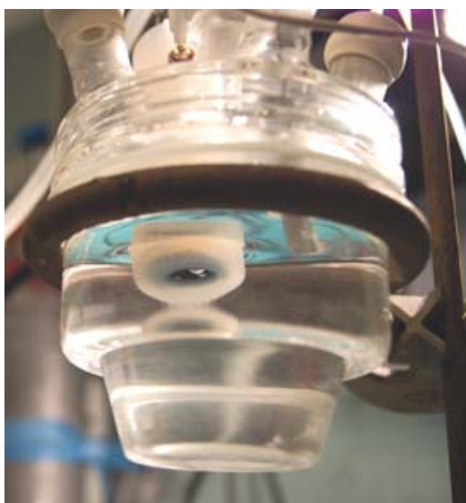
Electrochemical cell in half-cell configuration designed for testing the new catalysts with the technology developed at the Liten Institute.
