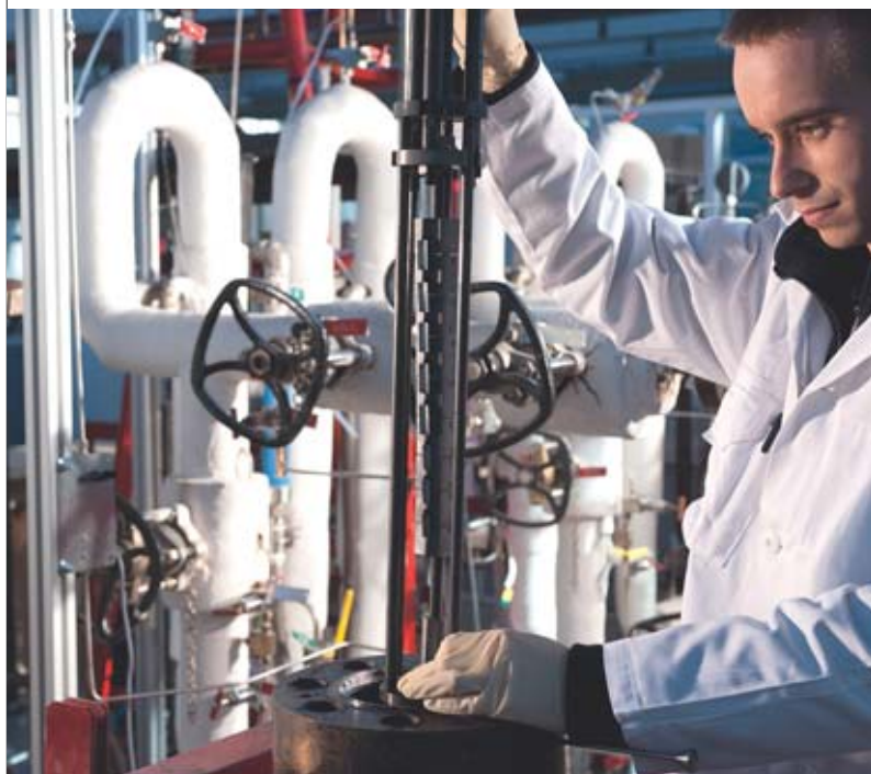
Placing stress corrosion samples in the Vénus facility in the Saclay Center.
