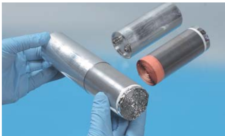
Left, production of positive composite electrodes using the solvent method. This process entails the production of an "ink" by dissolving an organic binder in a liquid and dispersing solid particles [active material and additives] in this mixture. This ink is then coated on the metal collector, dried and calendered to reduce its porosity. Right, wound Li-ion storage batteries.
