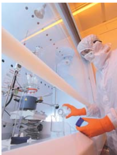
Surface modification in a clean room by liquid-phase silanization on a solid medium.
