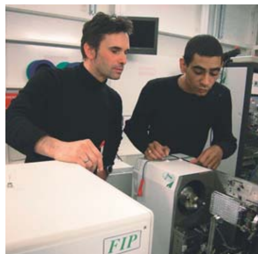
X-ray crystallography experiment at the ESRF, on the FIP (French beamline for Investigation of Proteins). This platform of the Partnership for Structural Biology, in Grenoble, is partly funded by the CEA. This beamline can in particular be used to evaluate the diffraction quality of very small protein crystals, without extracting them from their crystallization box (visible at bottom right).
