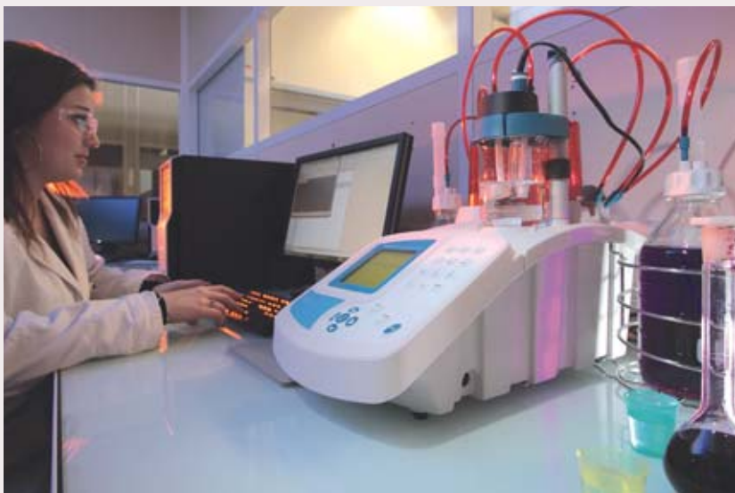
Physico-chemical characterization of a leachate obtained after dissolution of Li-ion battery active materials.
