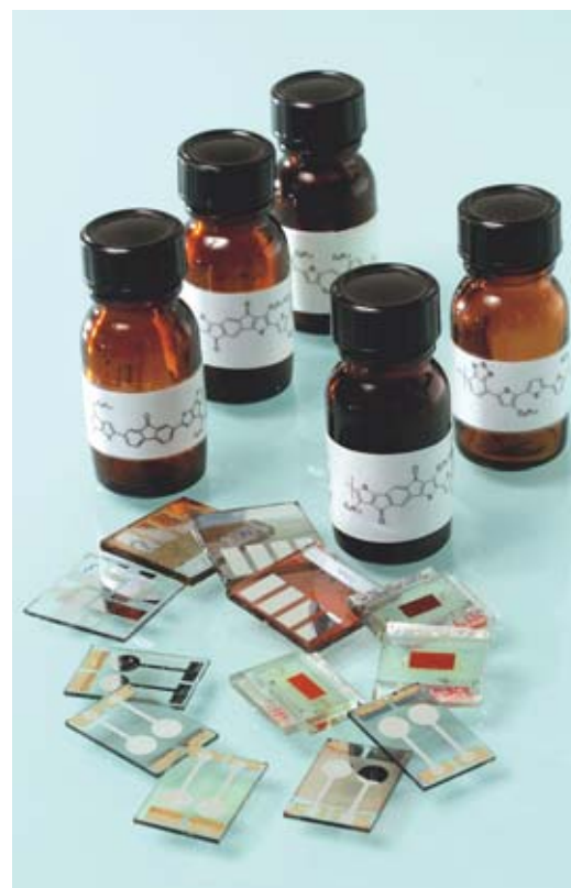
Samples of pi-conjugated polymers and photovoltaic cell test prototypes manufactured from them.
