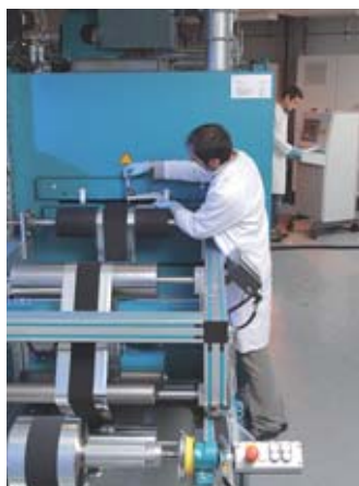
Left, production of positive composite electrodes using the solvent method. This process entails the production of an "ink" by dissolving an organic binder in a liquid and dispersing solid particles [active material and additives] in this mixture. This ink is then coated on the metal collector, dried and calendered to reduce its porosity. Right, wound Li-ion storage batteries.
