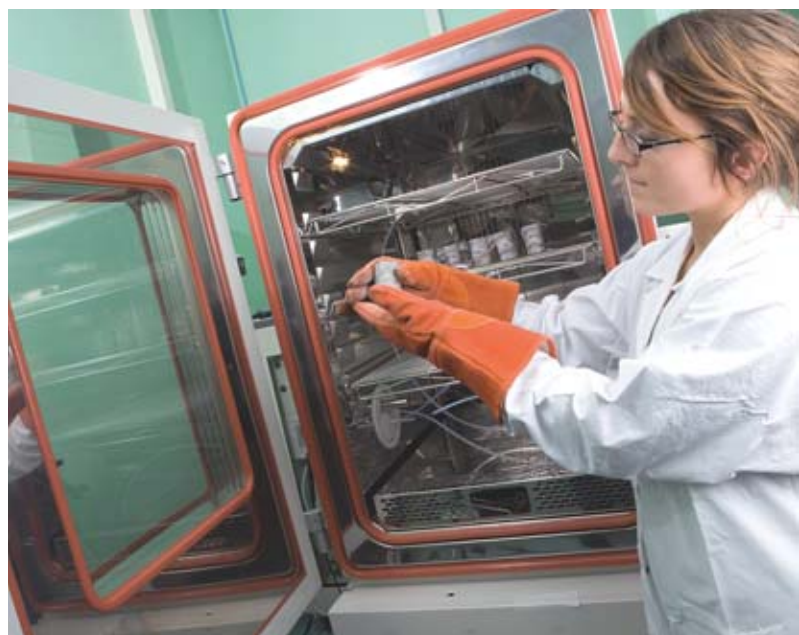
Study of concrete reactivity to CO 2 gas: performance of an accelerated carbonation test.
