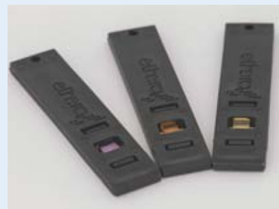
Exposure badges comprising nanoporous materials.
